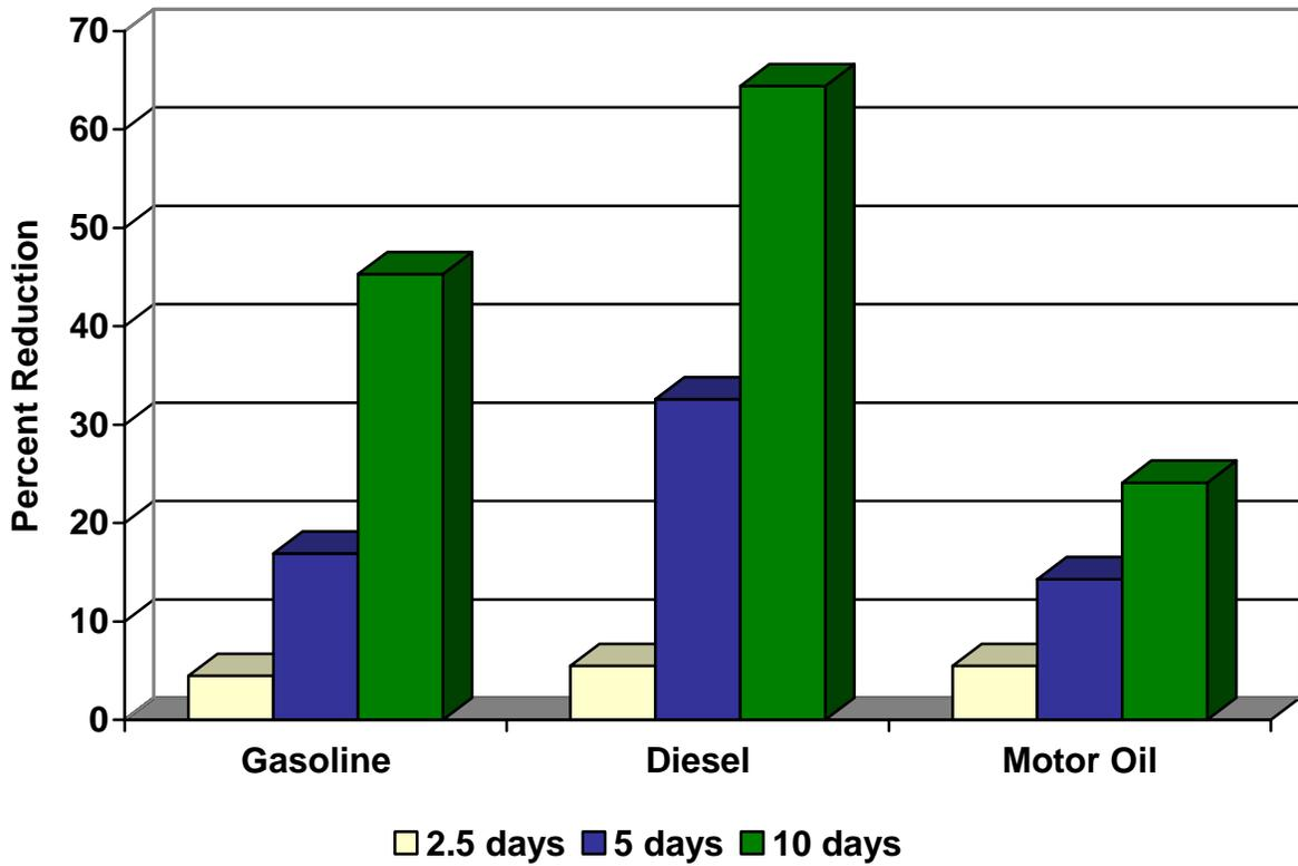
Figure 3 – Reduction of BTEX in Gasoline by Bacterial Strains in TRBC-200L
